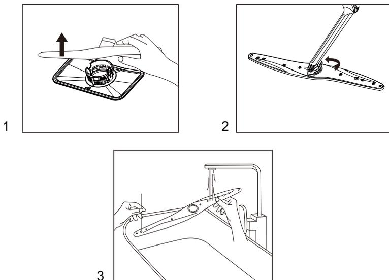
1. Pull the lower spray arm upwards to remove it.
