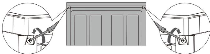
Remove the two screws at the back.
